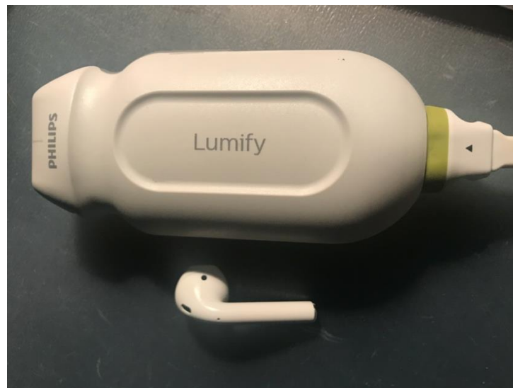
Fig.1 The core of the Lumix system, enclosed in a probe with a high level of miniaturization
