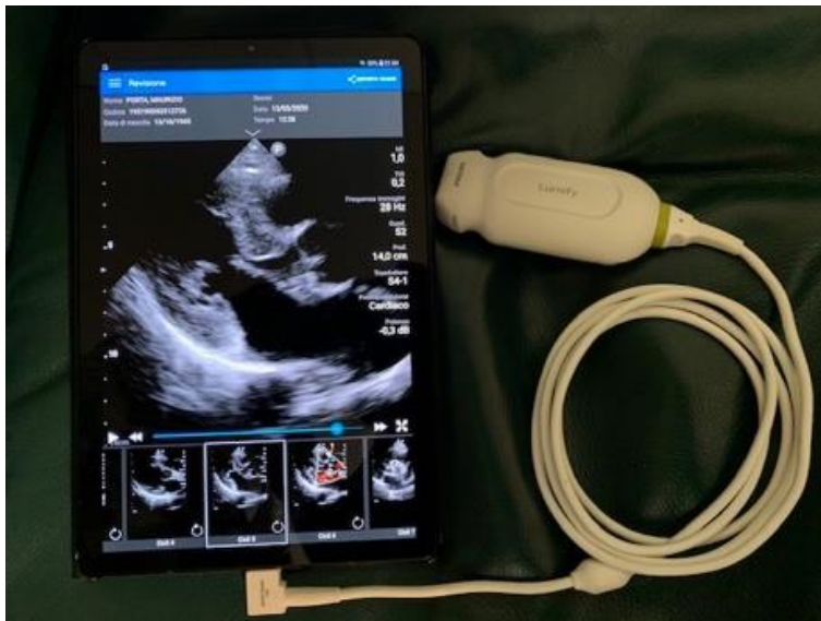
Fig.2 The probe can be connected to any handheld device, smartphone or ,as in this case, tablet.
